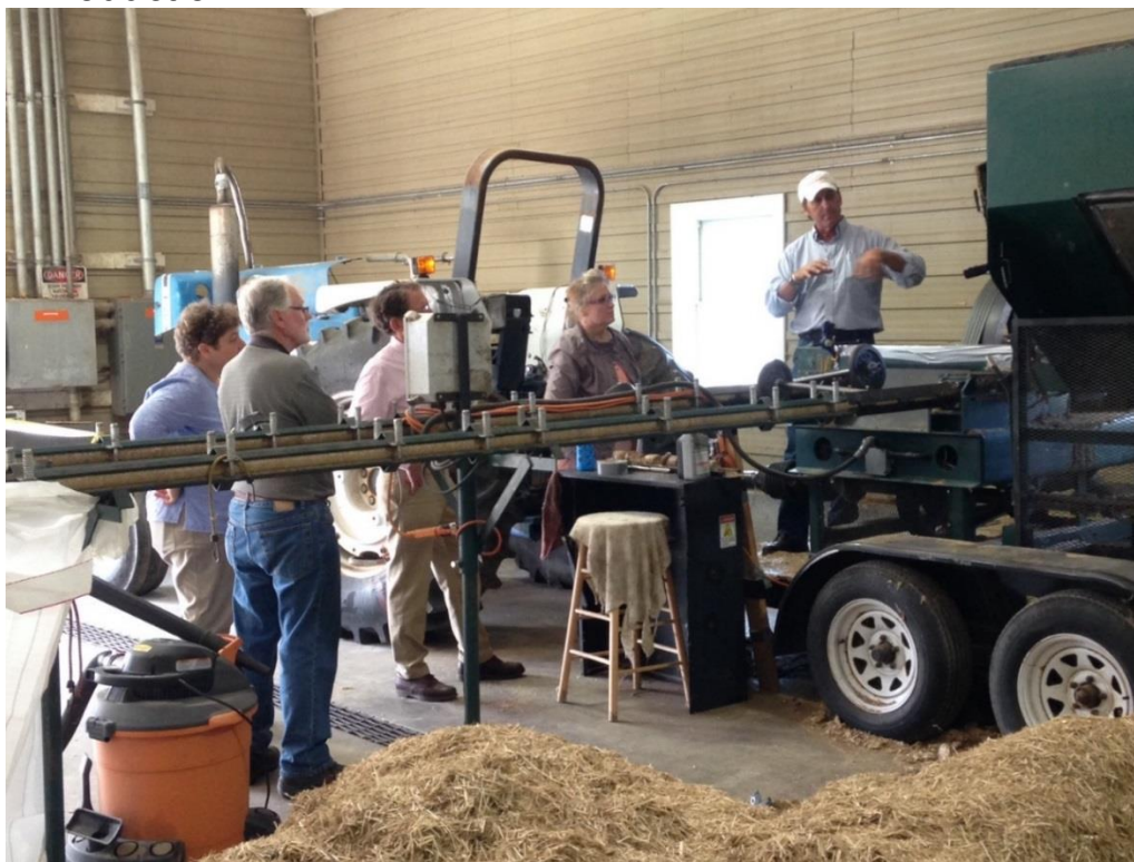
Figure 16 Adam Dantzscher explains biomass densification equipment (BHS "Slugger"), August 2015
