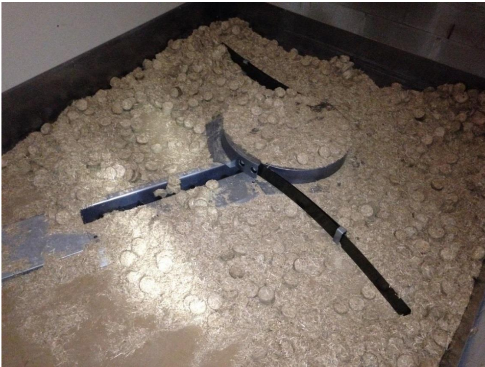
Figure 19 Evoworld chip conveyor in fuel bin, 2" puck fuel, 2015
