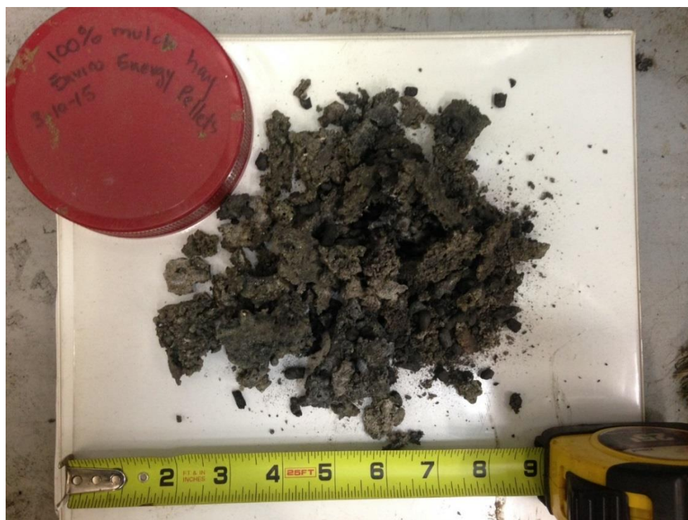
Figure 33 Enviro Energy hay pellets, clinker, 3-10-2015
