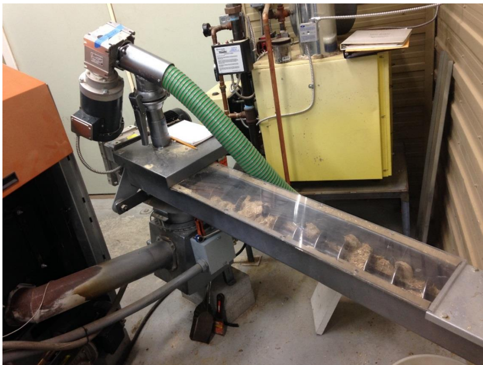
Figure 20 Evoworld HC 100 wood chip conveyor loaded with 2" pucks, March 2015
