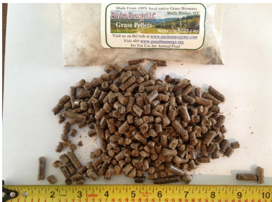
Figure 25 Enviro Energy 1/4" Diameter mulch hay pellets
