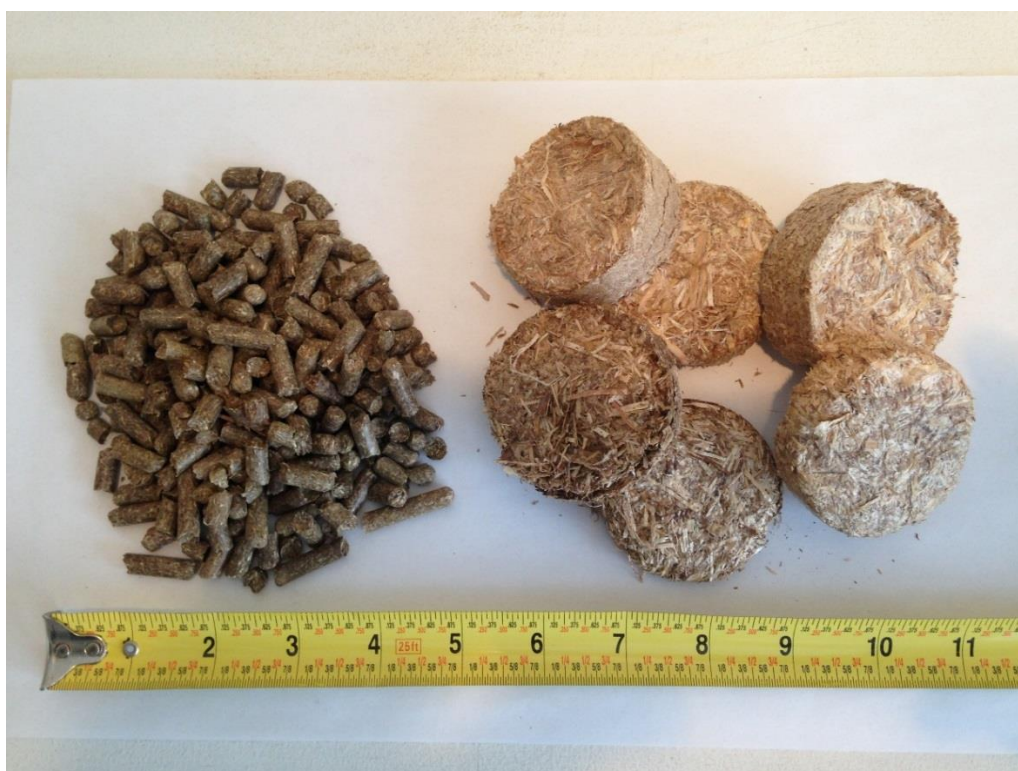
Figure 17 1/4" diameter pellet form and 2" diameter "puck" form
